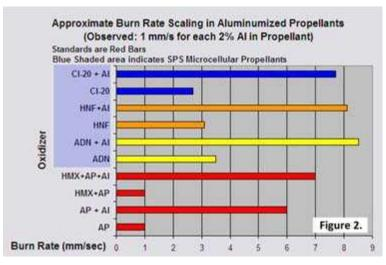
significantly reduce the need to use Aluminum for burn rate control altogether. Problems associated with Aluminized propellants such as particulate exhaust pollution, nozzle erosion, two-phase flow, and pooling of aluminum melt in the engine could be significantly reduced or completely eliminated.
