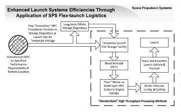
**location**, **even at the launch site**. These microcells flow like low-viscosity fluids, and are easy to pour and pack in an engine mold of any dimensions, then infused with a low-viscosity binder polymer, and, cured into a solid monolithic propellant grain using either UV irradiation or thermal curing.
